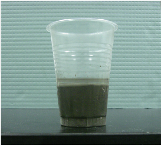
Fig. 5. Leakage of paraffin in the thermal energy storage composite.
